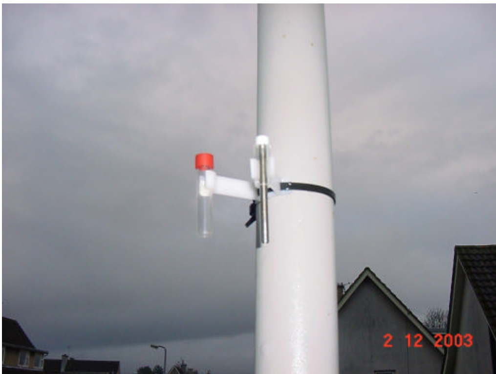
Monitoring equipment: Tenax and NO 2 diffusion tubes
