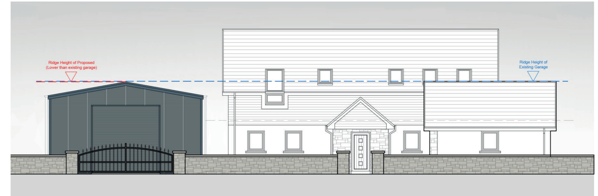
*Streetscape and Indication of Ridge Line Relative to Existing Garage*
