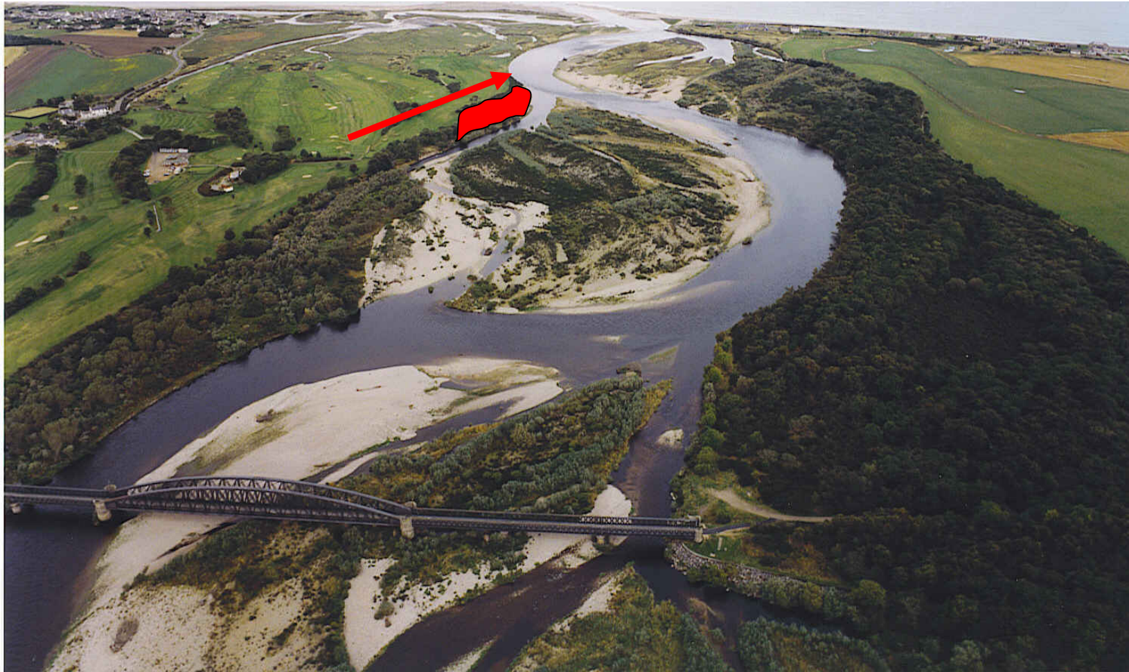
Plate 3 Arrow marks the area where Garmouth Golf Club is currently experiencing major bank erosion and the loss of their 17 th /18 th hole. The area highlighted in red is the approximate area lost since this photo was taken in 2000, due to development of meander loop through bank erosion coupled with the active back channel.
