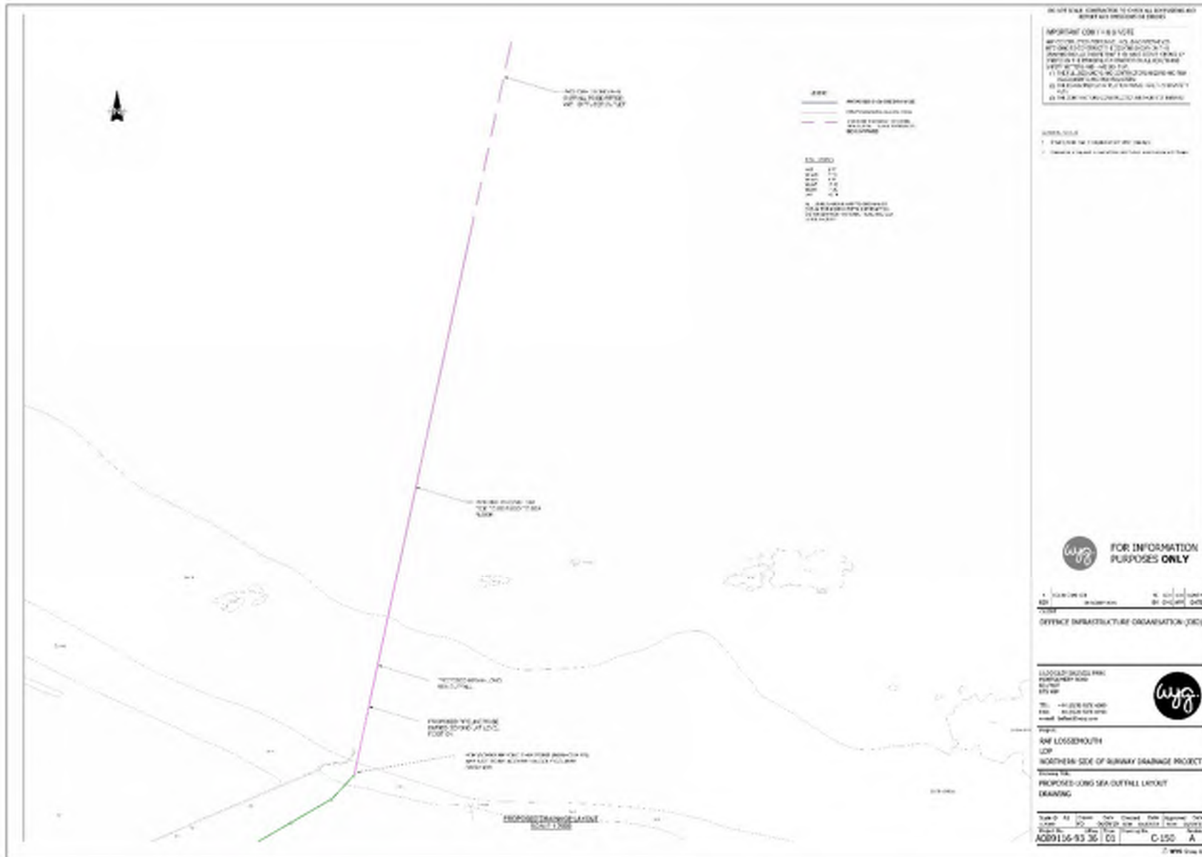
Figure 2. Chart showing the proposed drainage solution for the RAF Lossiemouth Development, including the long sea outfall (marked in pink).
