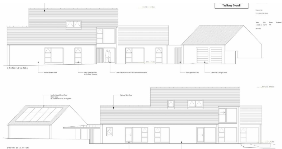
Figure 1 - elevations of neighbouring approved replacement house
