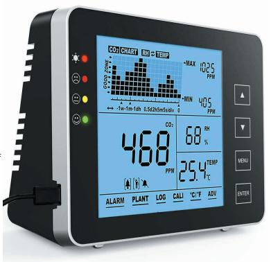
The sensor should be located in a reasonably central location. Not directly in front of an open window and not in a stagnant area right up against a wall. It will need to be near a power supply.
