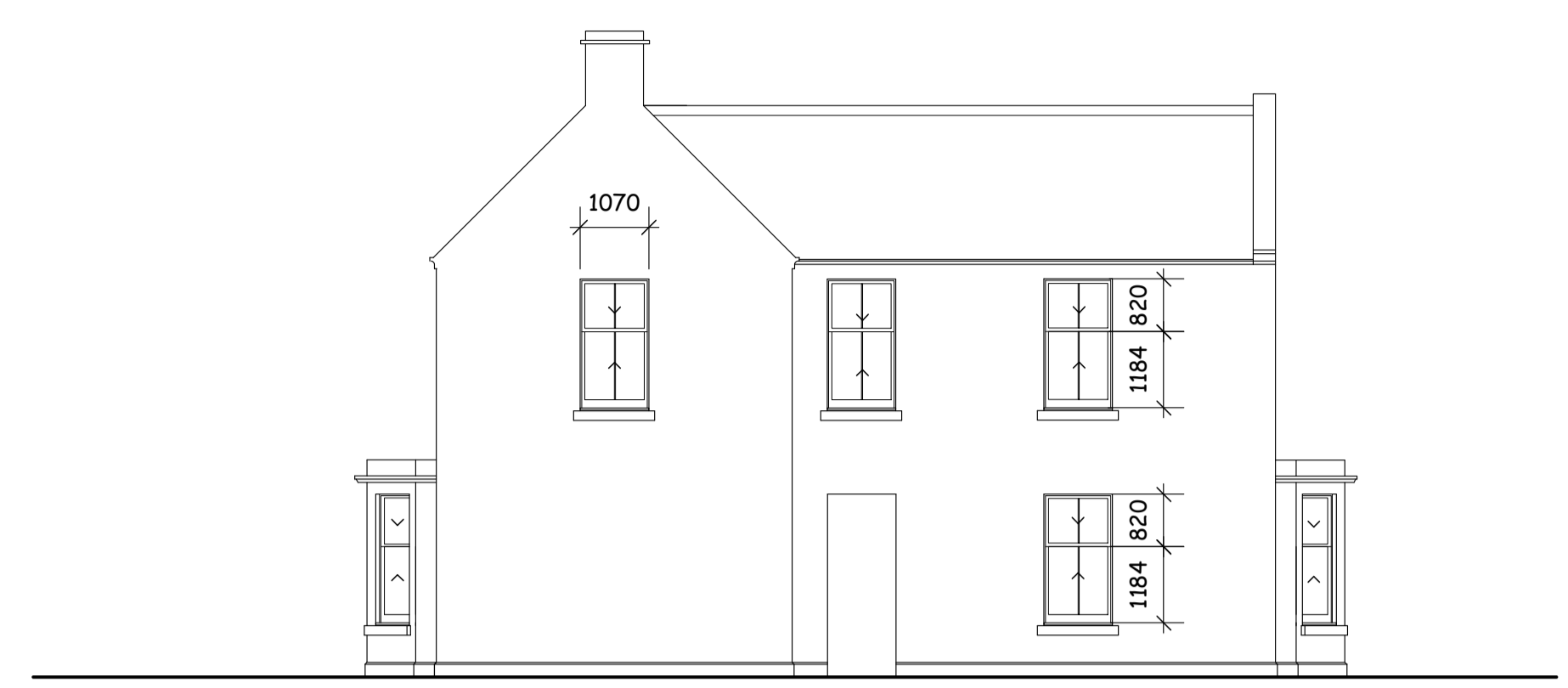
Existing West Elevation 1 : 100
