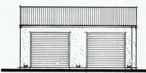
Front elevation 1-100 •2 No 3.6m wide by 3.2m high roller shutter door to frontage
