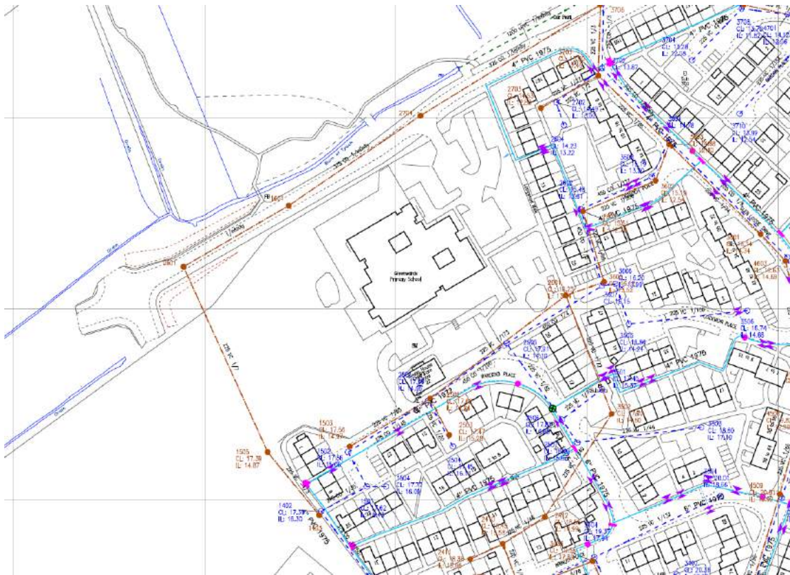
Figure 3-3. Public sewers and water mains around the residential area and primary school to the east of the site.
