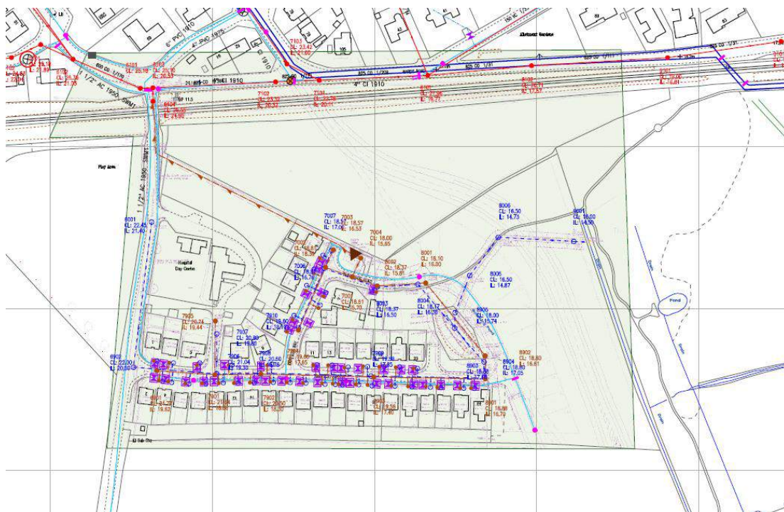
Figure 3-2. Public sewers and water mains around residential area in the north of the site. Note surface water sewer discharging east to land drain system.
