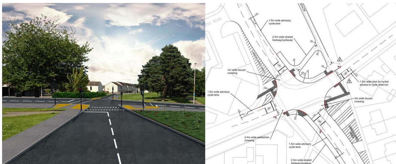
Figure 7.10 - Visualisation and Technical Drawing of Revised Junction
